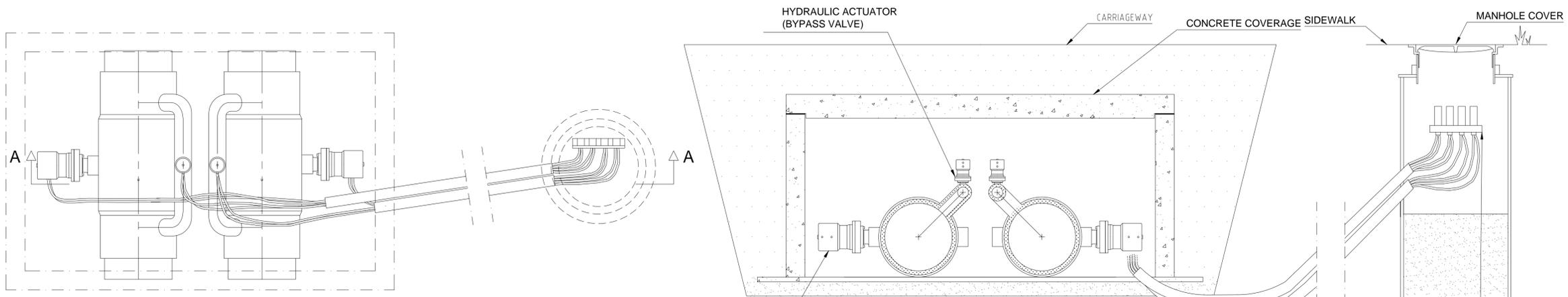
**PREINSULATED VALVE WITH HYDRAULIC ACTUATOR AND BYPASS VALVE**
