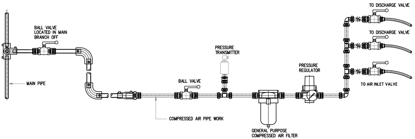
DETAIL 1: COMPRESSED AIR SYSTEM TYPICAL ASSEMBLY DETAIL FOR DV ROOM
