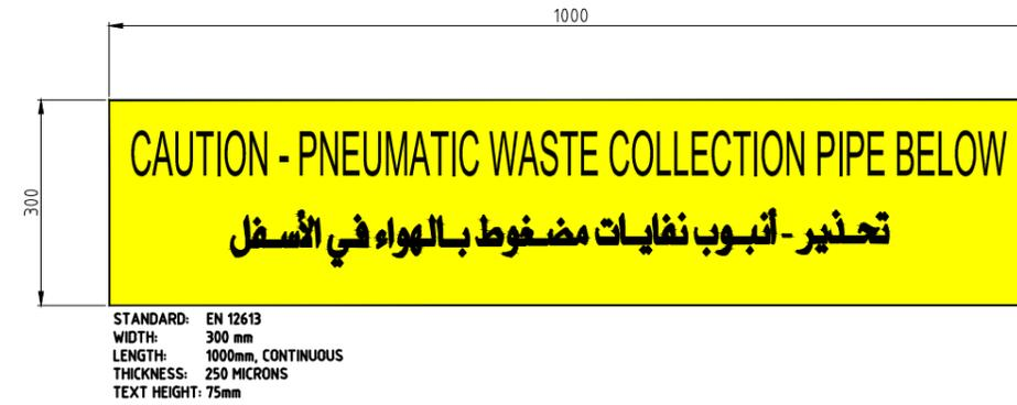
DETECTABLE WARNING TAPE FOR UNDERGROUND PWC PIPE
